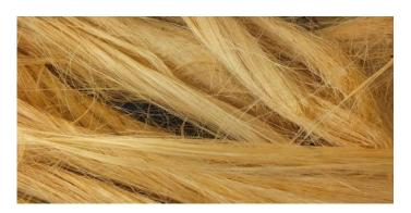
Banana Plant is an auspicious and ancient fruit crop grown in the South of India. After the fruit and the leaves are harvested, the bark of the tree is used which otherwise would have gone waste. Banana Fiber is extracted from Banana tree bark. The trunk is peeled. Brown-green skin is thrown away retaining the cleaner or white portion which will be processed into knotted fibers.
